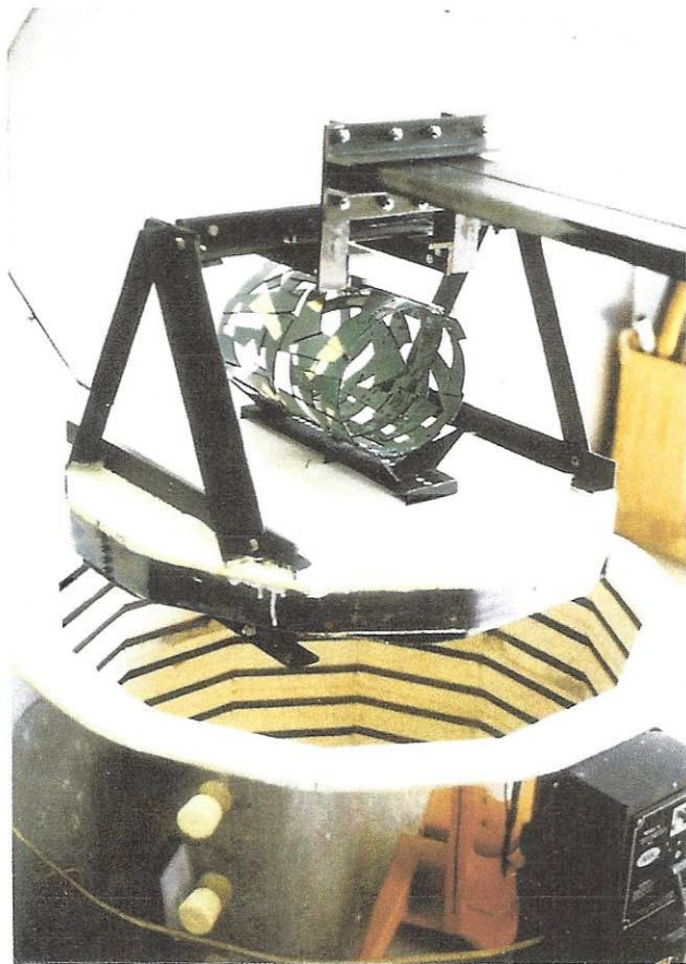
Work is positioned over opened, hot kiln.
