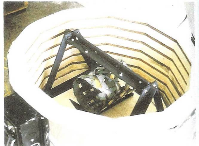
After work is inserted into kiln, the lift truck is backed away from the kiln and the lid is closed. The firing lasts approximately 30 minutes.
